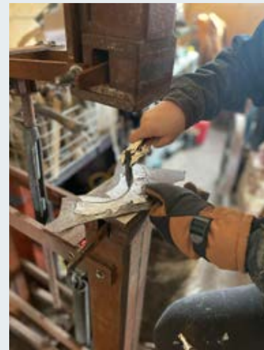
Making frame with Treadle Hammer. Photograph by Christopher Rantala.
